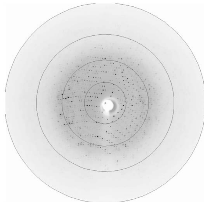
Figure 2 The first diffraction image from the native NiR crystal at room temperature. Diffraction spots are seen to 1.8 Å in the initial images; however, the crystal rapidly decayed. The unit-cell parameters of the room-temperature data collection were slightly larger than the frozen crystals. Resolution rings are 6.0, 3.0, 2.0 and 1.5 Å.
